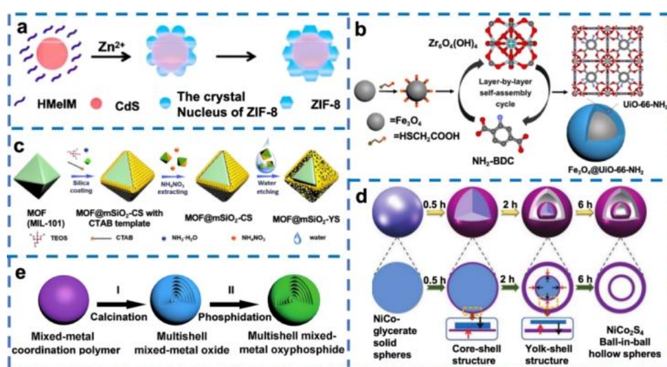
Figure 7 Schematic preparation of (a) CdS@ZIF-8 core-shell structure; Reprinted with permission. Copyright 2016, Springer Nature; (b) Fe_3O_4@UiO-66-NH_2 core-shell
