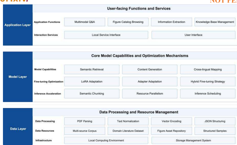
Figure 1. Architecture of the locally deployed multimodal literature model system. Q&A: question answering; LoRA: low-rank adaptation.
